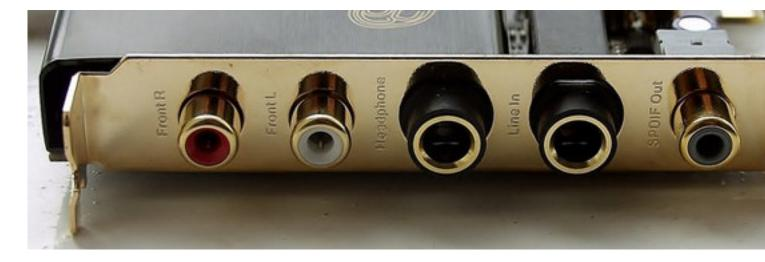
The analog output (cinch) and SPDIF (coaxial and optical via an adapter) can work simultaniously on the 432 EVO ESSENCE.
